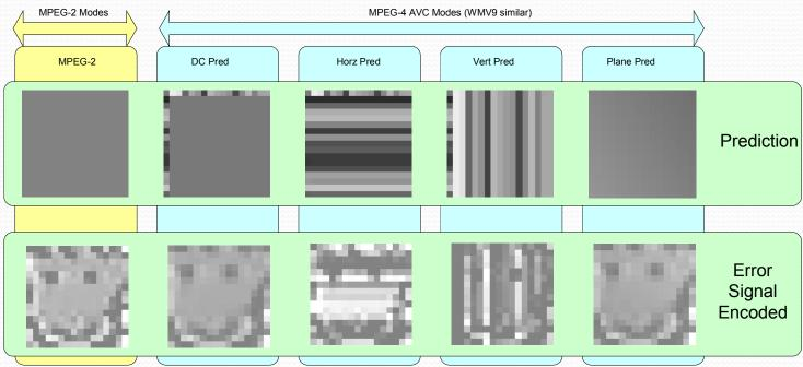
In AVC, adjacent blocks can be used to encode the current block and reduce the error signal
