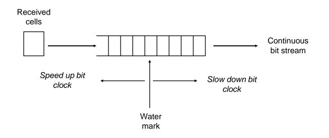
• Local clock is provided by a phase-locked loop driven by the buffer fill level.
