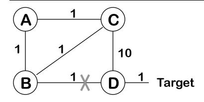
Routes to Target: A: route via B, distance 3 B: route via D, distance 2 C: route via B, distance 3 D: direct, distance 1
